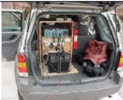
Rear view of rack with deep cycle battery & pump system feeding the analyzers.
