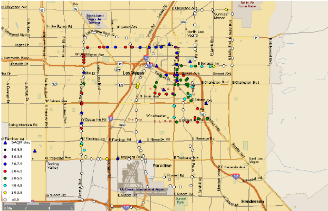
Figure 6-10 Observed CO Concentrations (ppm) During December 18 Morning Period
