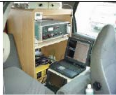
View looking from front seat to the back instrument rack, inverter & computers.
